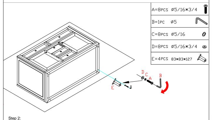
Attach the Legs to the Cabinet, insert the bolt (A) through the Spring Washer (C), Flat Washer (D) through into the pre-drilled holes at the bottom of Cabinet, then tighten the bolts using by Allen Wrench.
