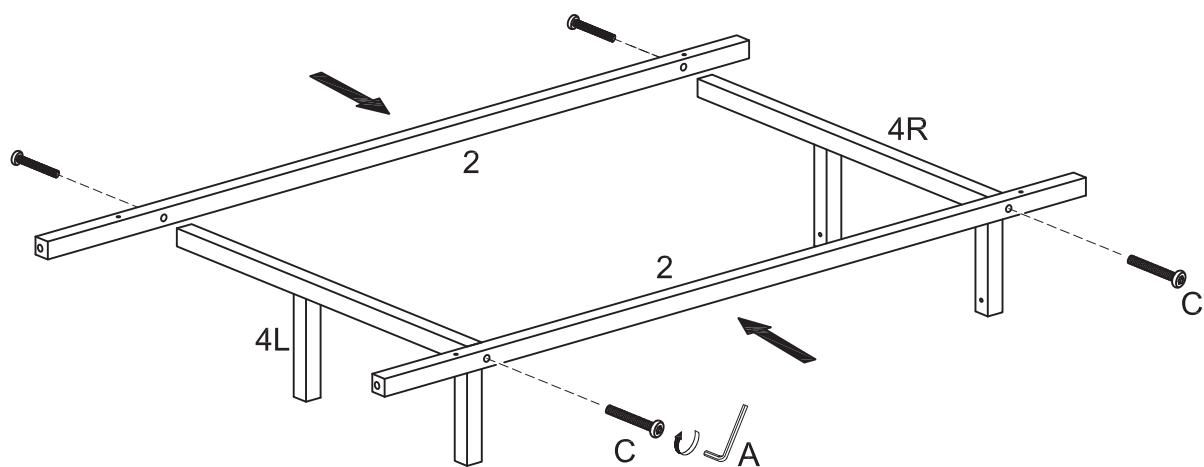
Attach upper crossbars (2) to keyboard tray supports (4L) and (4R) using medium bolts (C). Note the proper alignment of all bolt holes as shown above. Tighten medium bolts (C) with wrench (A).
