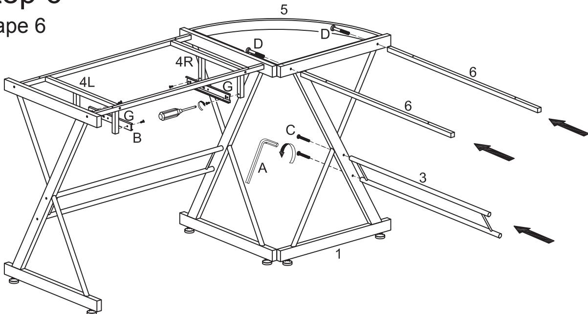
Attach the tray arms of keyboard tray sliders (G) to keyboard tray supports (4L) and (4R) using short bolts (B). Ensure that the open end of each tray arm is near the front of the desk. Tighten short bolts (B) with a screwdriver. Attach leg (1) and crossbars (6) to corner frame (5) using long bolts (D). Attach lower crossbar (3) to leg (1) using medium bolts (C). Tighten all bolts (C,D) with wrench (A).
