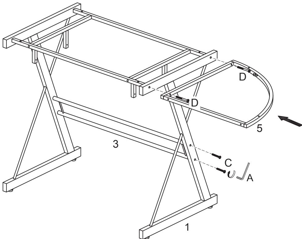
Attach leg (1) and corner frame (5) to the assembly from the previous step using long bolts (D). Ensure that the glass supports of corner frame (5) are facing up (reference Steps 8 and 9). Secure leg (1) to lower crossbar (3) using medium bolts (C). Tighten all bolts with wrench (A).
