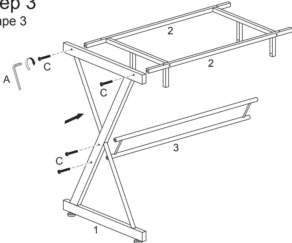
Attach upper crossbars (2) and lower crossbar (3) to leg (1) using medium bolts (C). Tighten medium bolts (C) with wrench (A).
