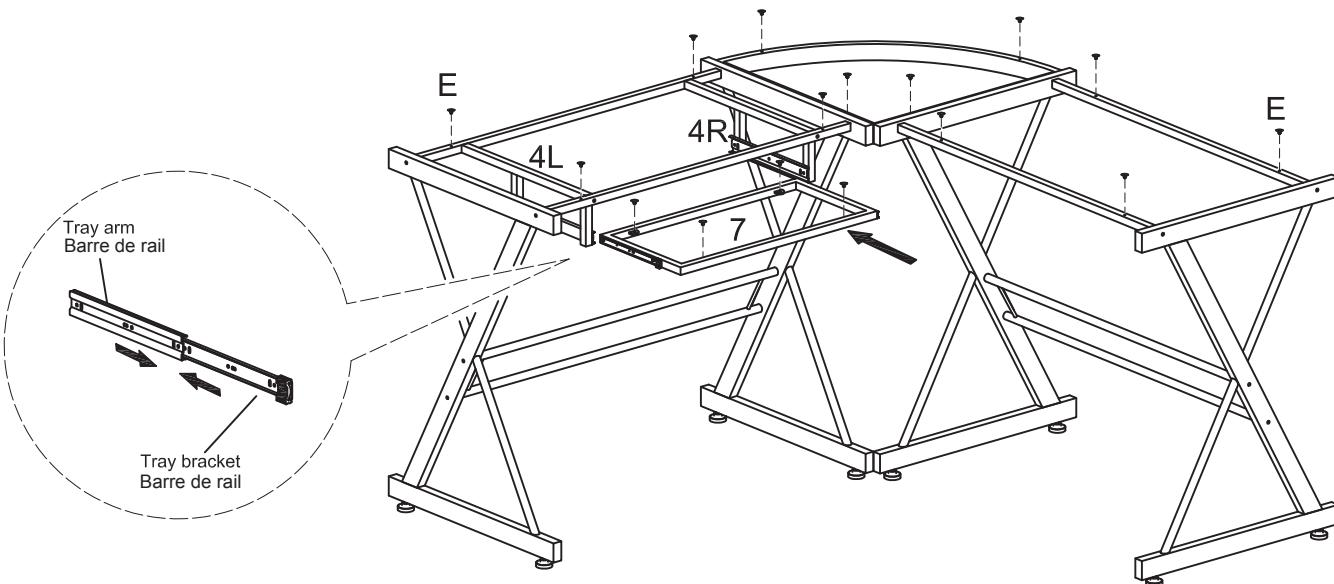
Carefully slide keyboard tray frame (7) into place. The tray brackets attached to keyboard tray frame (7) will slide into the tray arms attached to the keyboard tray supports (4L) and (4R). Insert rubber suction cups (E) into the desk frame as shown above.
