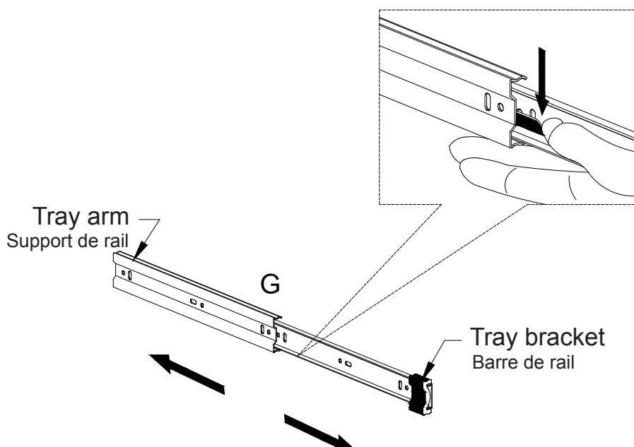
Disassemble keyboard tray slider (G) by sliding the tray arm and tray bracket apart. Depress the small lever of the tray bracket and carefully pull the two pieces apart. Repeat this process for both keyboard tray sliders (G).
