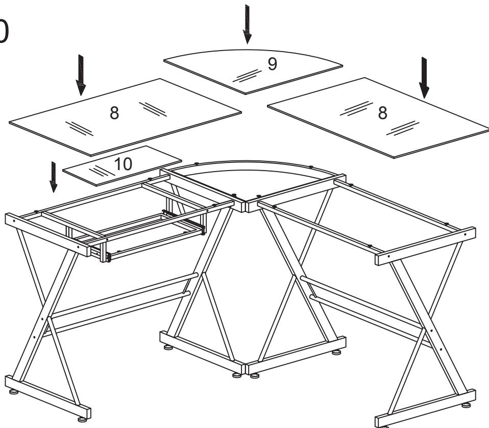
Carefully lay keyboard tray glass (10) in place and gently press to secure. Carefully lay glass (8) and corner glass (9) in place and gently press to secure.
