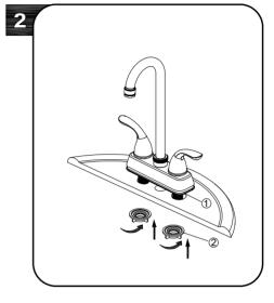
Place gasket (1) on bottom of new faucet. Place faucet through mounting holes in sink. Secure faucet to sink using mounting nuts (2) provided.
