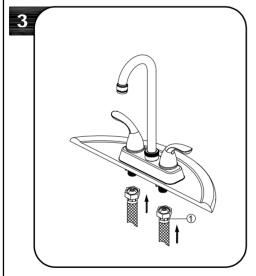
Make connections to water lines. Use 1/2" IPS faucet connections (1) Use wrenches to tighten connections. Do not overtighten.
