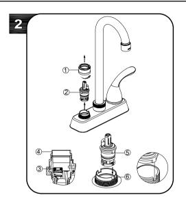
Shut off water supply.Remove handle(refer to step 1).Loosen bonnet (1) by turning it counter-clockwise and lift out the cartridge (2).Inspect the rubber valve seat (3) inside body (4).Make sure the wings (5) on the two sides of the cartridge bonnet fit well into the slots (6) on the body.Tightly bonnet (1).Reinstall the handle.
