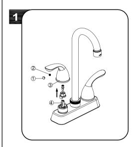
Turn off water before proceeding! Remove index(1). With valves in "closed" position,unscrew fastener (2) and remove handle (3) from valve stem (4).
