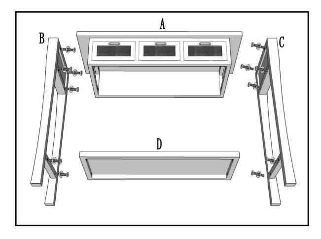
**Step 1**Attach the legs (B), (C) to the table top (A), use allen key to tighten the bolts(E). Then attach the shelf (D) to the legs, tighten all the bolts(E).
