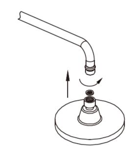
**12.** Install the rain shower head. Make sure to use a sealing washer.
