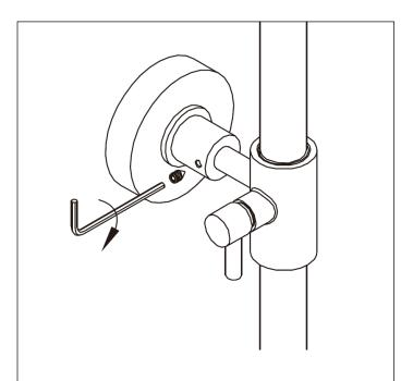
**11.** Slide the shower set into the mounting bracket and secure into place with the set screw.
