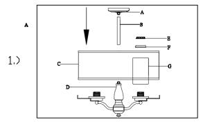
Step.1: Attach glass (G) to fixture using socket ring (E) and spacer (F) to secure. Add medium base bulbs. Attach shade to frame using screws. Run wire through stem (B) and canopy (A), then attach to fixture (D).
