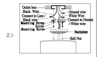
Step.2: Remove mounting strap from fixture and install to electrical box. Wire fixture to wires in outlet box. Copper wire is for Ground. Attach fixture to mounting bracket using ball nuts to secure.
