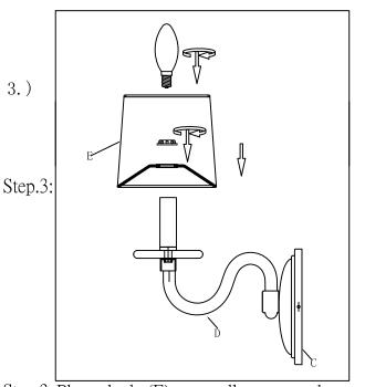
Step.3: Place shade (E) on candle cover and secure using screw ring provided. Then, install 40 Watt candelabra base bulb.
