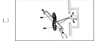
Step.1: Remove mounting bracket (A) from back plate (C) and install to electrical box.
