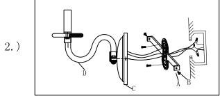
Step.2: Install fixture to mounting backet (A) using back plate screws (B).
