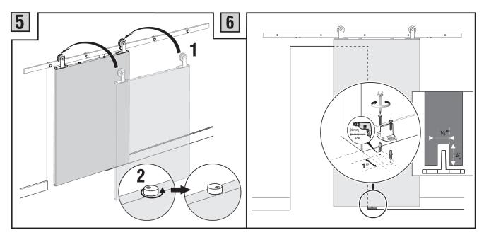
Attach the door to the rails making sure that the anti-jump disks are engaged to avoid a serious accident.
