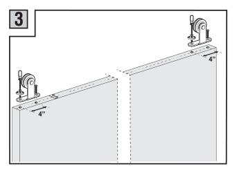
Drill holes in the top of the door 4" from the edge as pictured to accommodate the door rollers. The bottom of the doors should be routed at this time in order to accept the floor guide.
