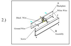
Step.2: Wire fixture to wires in outlet box. Copper wire is for Ground. Attach LED assembly (B) to the backplate (A) using screws (D) provided.
