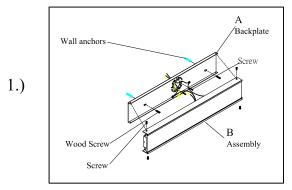
Step.1: Remove backplate (A) from fixture (B) and install to electrical box. Mark where anchors meet the wall. Drill holes using 3/16" ± drill bit where marked. Install backplate (A) to outlet box and attach anchors to secure bracket at ends.
