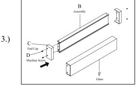
Step.3: Use end caps (C) to install glass (F) to the assembly (B) and secure with machine screws (D) provided.
