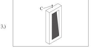
Step.3: Caulk around fixture with outdoor silicone sealant to prevent water intrusion. Leave a small gap at the bottom to allow moisture to escape. Install fixture to mounting bracket (A) and tighten mounting screws (C).
