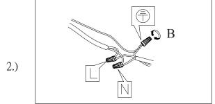
Step.2: Wire fixture to wires in outlet box. Green/Copper wire is for Ground.
