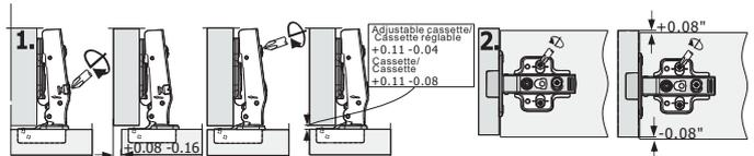
1. Adjusting screws on the hinge arm can adjust the front and rear of the door panel
