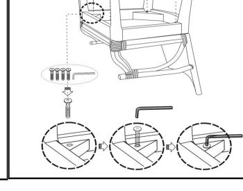
Assembly part A and B with Nuts and tighten with L key
