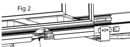
Press release lever behind side skirt on each side by sliding up or down depending on which side. Unit will separate when both levers are disengaged.
