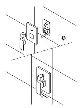
7. Install the spout.(wrap the PTFE tape on the thread).
