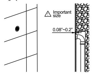
5. Install the hand shower bracket. (wrap the PTFE tape on the thread).
