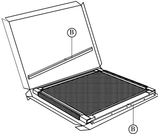
STEP 2 : Attach Mirror Support Rail ( B ) to Mirror ( A ) as shown and tighten with CSK Screw ( 1 ).
