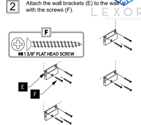
IMPORTANT: Consult an expert for the proper screws/bolts to use when attaching to various constructions. Screws provided do not attach to all wall construction types. Anchors are not required if brackets are installed in stud.
