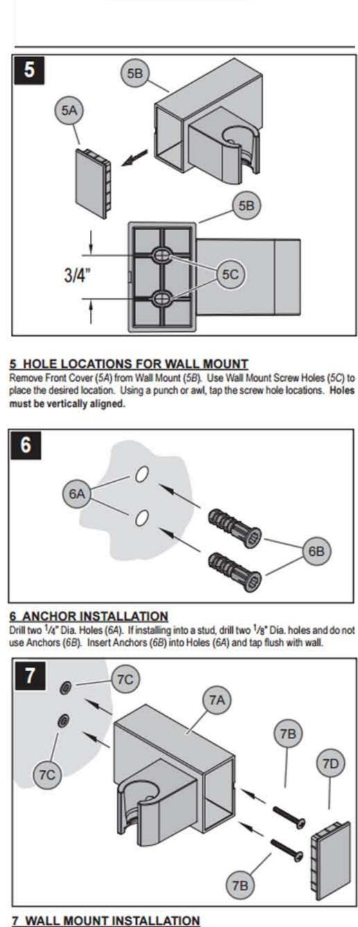
Place Wall Mount (7A) onto wall and insert Mounting Screws (7B) through Wall Mount Holes (7C) and tighten until Wall Mount (7A) is flush with the wall. Do Not Over Tighten!
