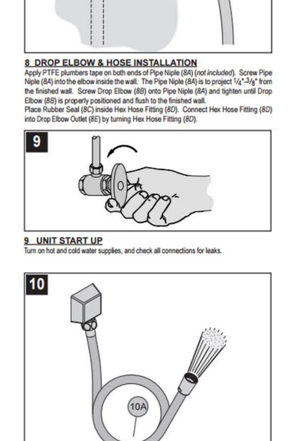
For final flushing, turn valve on and allow water to run through the Hose (10A) for several minutes. Allow water to run for several minutes untill all foreign matter clears the line.
