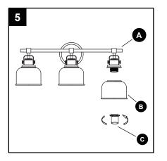
6. Install light bulb (not included). Use three standard-base bulb.
