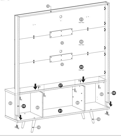
• Connect the Lower Panel (09) onto Middle Shelf (07) with dowels (D) and apply bolts 5.0 x 50mm (E) to fix the lower end of Columns (08) on the Base (01) and the Lower Panel (09) on the Middle Shelf (07).
