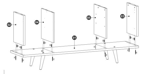
• Connect the Side Panels (02) and (03) and the Partitions (04) and (05) onto the Base (01) with dowels (D) and bolts (E).
