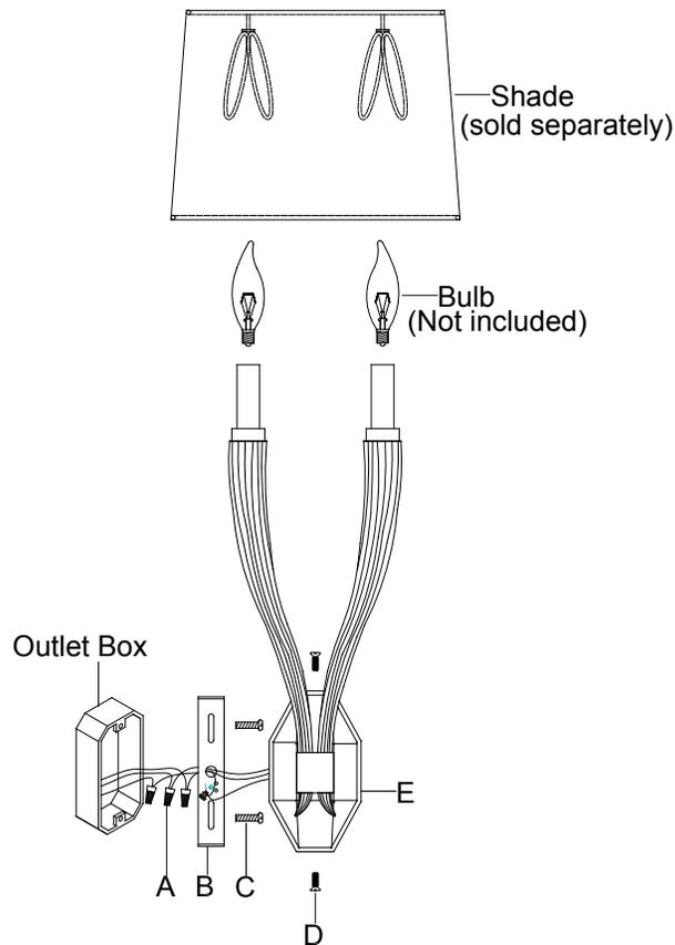
1. Carefully remove the crossbar (B) from the back plate(E) by removing side screws(D).
