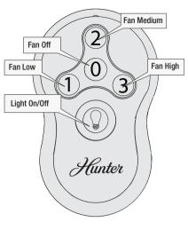
To turn on fan, press a fan speed button. Speeds range from off (0) to high (3). Quickly press the Light button to turn the lights off and on.
