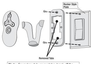
**Note:** For rocker-style cover plates, break off the tabs by pushing outward.
