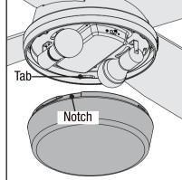
Lift the globe and align the notches in the globe with the tabs in the light kit. Attach the glass bowl to the light kit by twisting it clockwise until it snaps into place.
