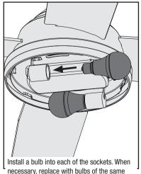
necessary, replace with bulbs of the same type and wattage.
