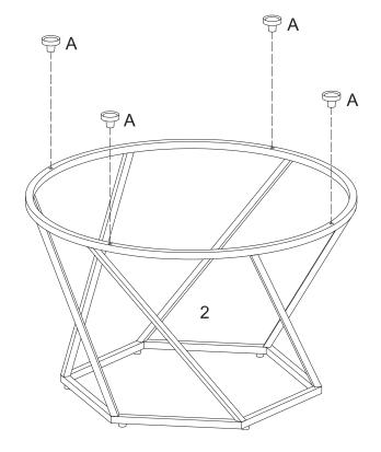
Insert the rubber suction cups (A) to the metal base (2).
