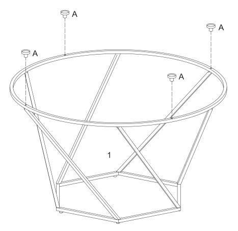
Insert the rubber suction cups (A) to the metal base (1).
