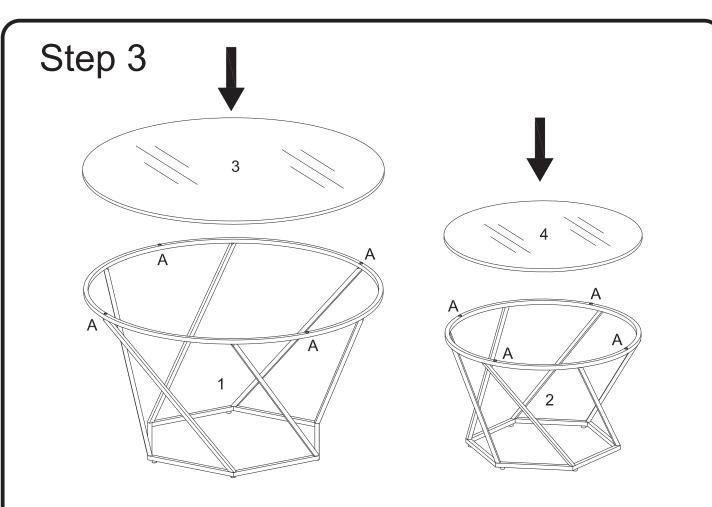
Place the glass table top (3,4) on top of the metal base (1,2) carefully as per diagram.
