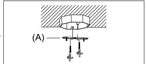
Step.1: Remove mounting bracket (A) from fixture and install to electrical box.
