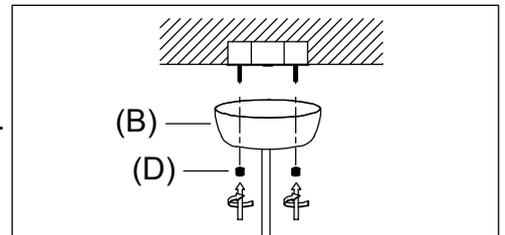
Step.3: Install body (B) to bracket (A) and secure with nut (D) . Screw glass (C) to the coupling. Install light bulb.
