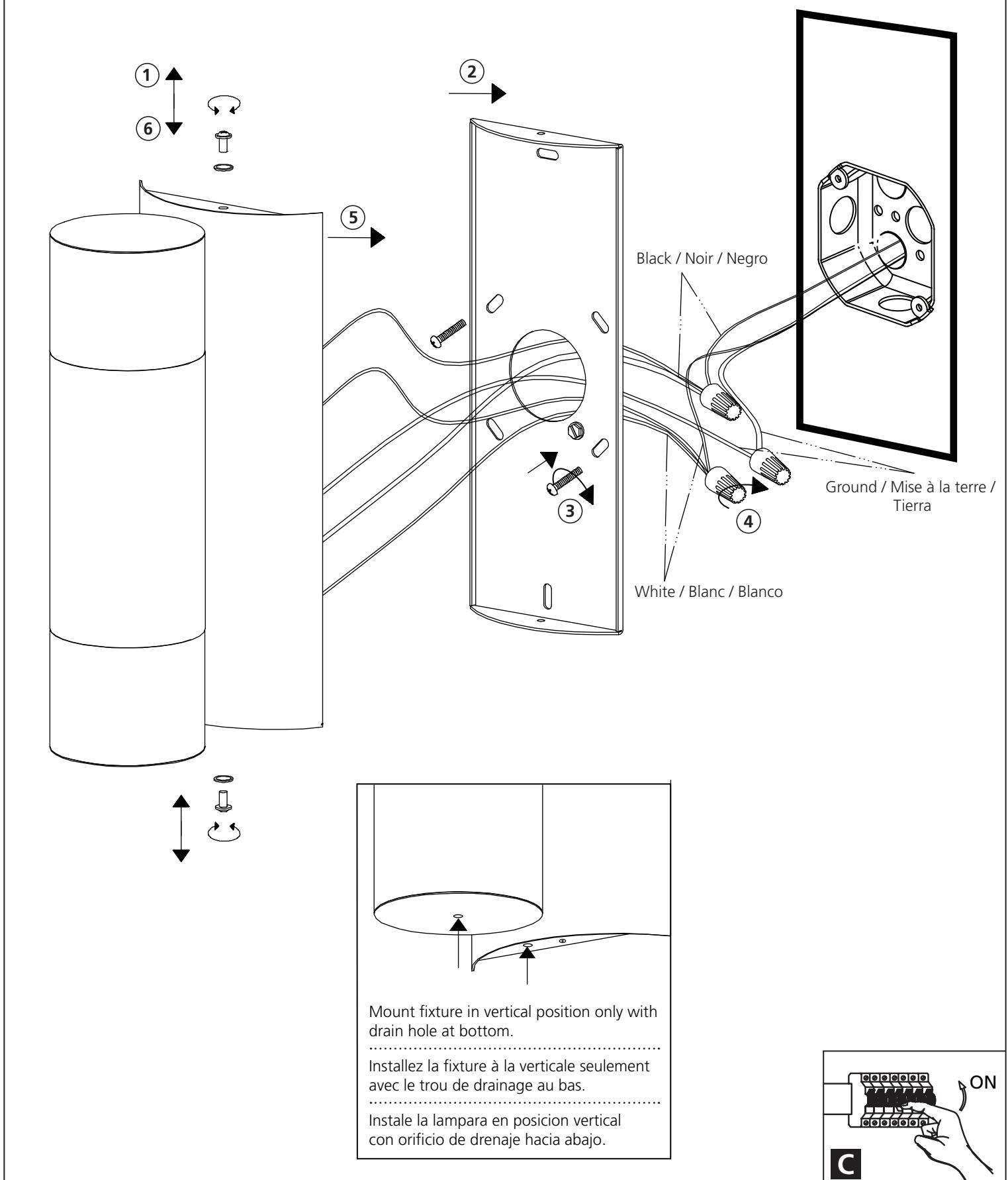
Mount fixture in vertical position only with drain hole at bottom.
