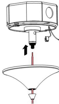
3. Position the "side collar" (supplied) so that a small section (1/16") of "braided cord" protrudes from the top of the collar.
