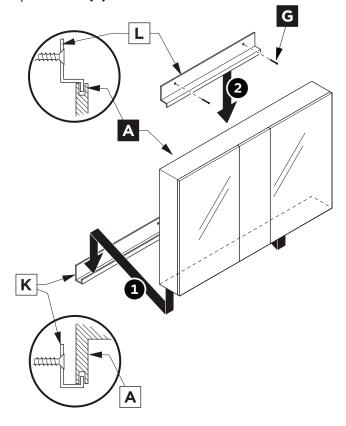
\*This step requires assistance to hold cabinet in place until top bracket is securely attached.
