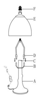
Step 1 Insert the Harp (D) into the Saddle (B). Put the shade(E) on the Harp(D), then tighten the Finial (F)into the Harp (D)
