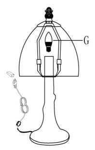
Step2 Insert the bulb(G) into the socket(C).
