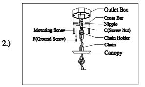
Step.1: Wire fixture to wires in outlet box.
