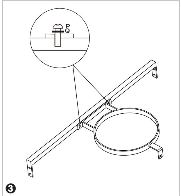
**4** Attach **Tank Support Bar 1** to **Door Frame Leg F** and **Support Leg 1 G** by aligning holes at each end of **Tank Support Bar** with holes at the bottom of **Door Frame Leg** and **Support Leg 1**. Place a **Washer Q** on each of four **Bolts P** and insert into holes. Tighten with **Hex Key X**.
