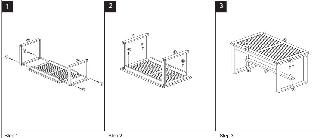
Attach front leg (B) to bar (A), using Allen bolt (D), tighten with allen key (H)
