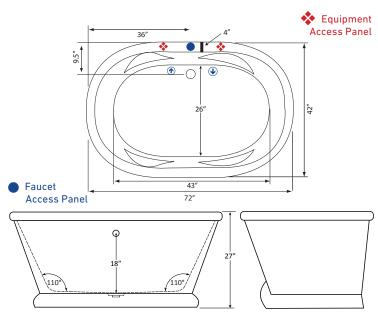
Decorative Pedestal is not on back side in order to accommodate equipment access. This side should be placed against wall.
