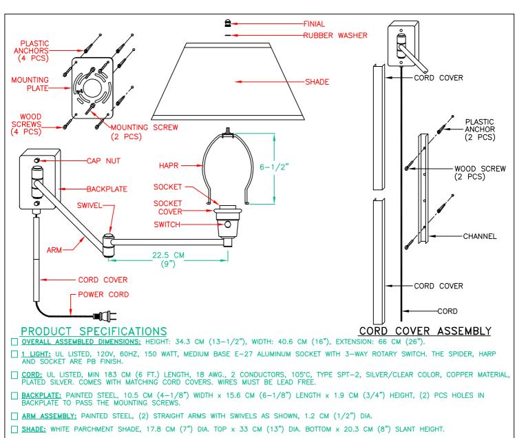
LABELS: UL, CSA OR CUL, MANUFACTURING DATE, MODEL # AND COUNTRY OF ORIGIN LABELS PROVIDED ON BACK OF WALL BRACKET. RELAMPING LABEL FOR 150 WATT MAX. 3-WAY TYPE "A" BULB PROVIDED ON SOCKET COVER.
