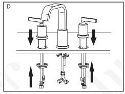
D. Slide hot and cold water handle / valve through mounting holes. Handles should point outward in off position. Secure the handles with the mounting nut. Hand tighten the nut onto the valve.
