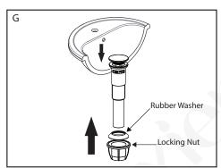
G. Remove rubber washer and locking nut from the drain assembly and slide the drain into the sink. Install the rubber washer first and tighten the locking nut to install the drain.
