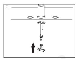
C. Insert the Tee connector to the center spout hose until it click in place. Make sure the hose is inserted fully until it lock in place. There will be an audible click when the hoses are connected properly.
