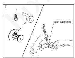
F. Apply Teflon (PTFE) tape on the shut off valves. Thread the tape in counter-clockwise direction. Use a wrench to tighten the hoses, by 1/4 turn. Please do not overtighten the connections.
