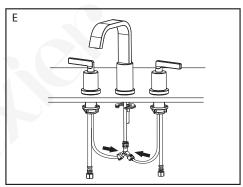
E. Connect the 2 supply hoses to the Tee connector. Make sure the hose is inserted fully until it lock in place. There will be an audible click when the hoses are connected properly.
