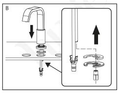
B. Place spout with flange through the center mounting hole on the mounting surface. Secure spout with C shaped rubber washer C shaped metal washer and locking nut.
