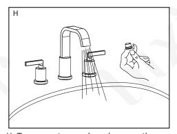
H. Turn on water supply and remove the aerator with a small coin or a flat head screwdriver and let the water run for about 1 minute to clear any debris in the plumbing system. Check for leaks at all connections. Reinstall the aerator to complete the installation.
