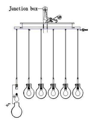
PLEASE USE TYPE"B" BULB MAX 25-WATT OR LED BULB MAX 5-WATT, THERE ARE 6PCS LED 4-WATT BULB IN THE BOX
