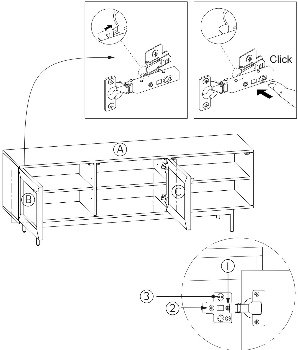
Attach Doors (B) and (C) using adjustable hinges on Top (A).
