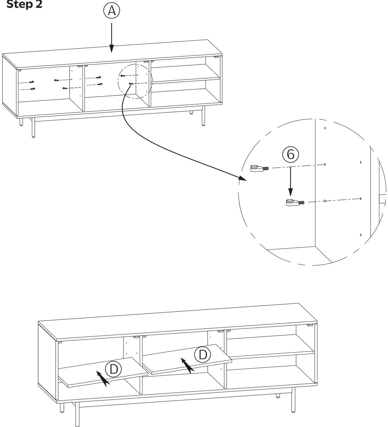
1. Insert Shelf Supports (6) into the holes in each cabinet of Top (A).
