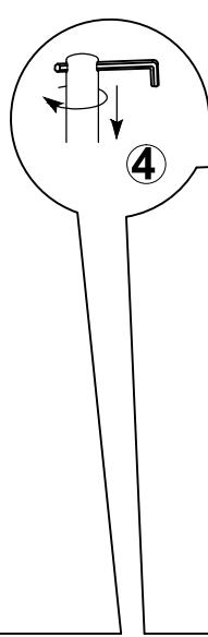
Insert Allan key through the holes to help tighten the poles.
