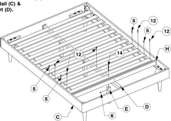
Bolt & screw the remaining Bed Slats (H) to the Side Rail (C).
