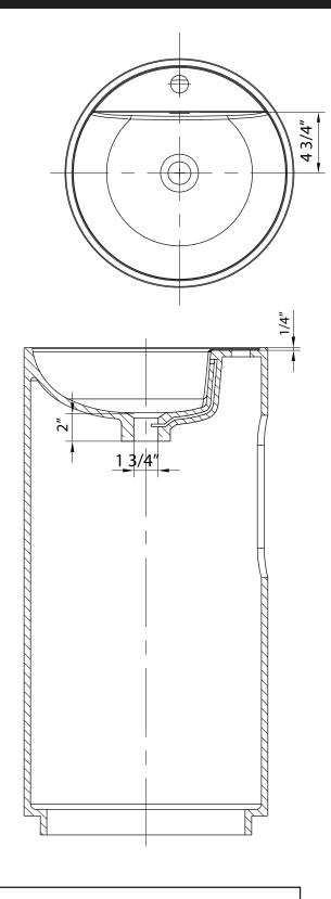
**ATTENTION!** Dimensions may vary by up to 3/8". It is highly recommended to pull all dimensions of actual model for installation and measuring purposes.
