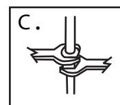
Tighten connection with two wrench to prevent damage to tube body.
