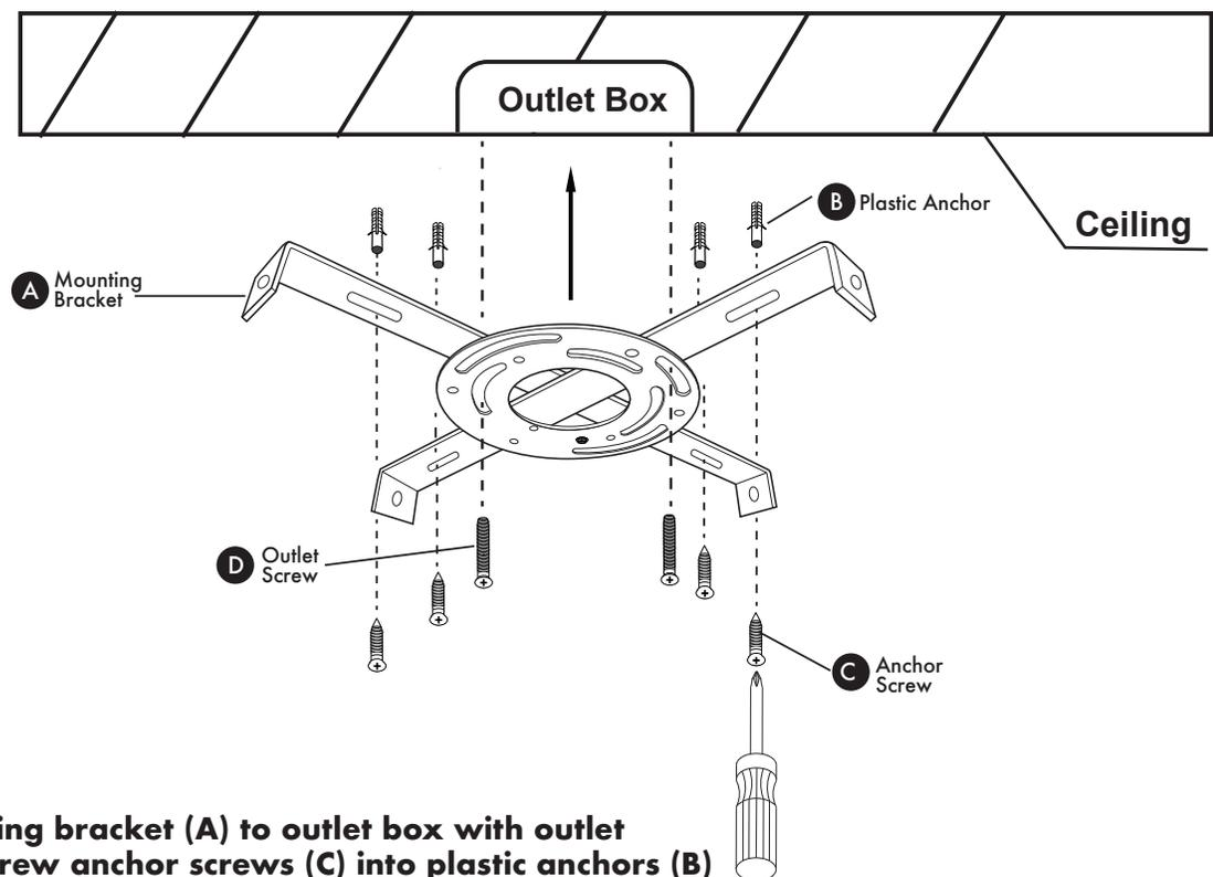
**Attach mounting bracket (A) to outlet box with outlet screws (D). Screw anchor screws (C) into plastic anchors (B) to secure mounting bracket (A).**
