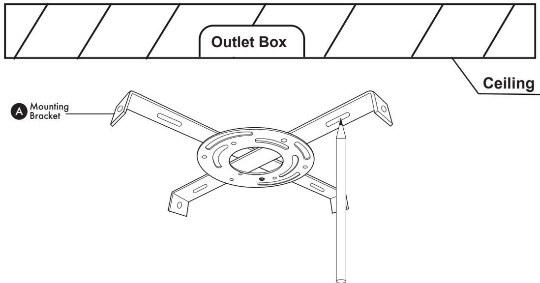
**Raise mounting bracket (A) to the ceiling. Mark location for the plastic anchors (B). Use drill to drill holes for plastic anchors (B). Insert plastic anchors (B) into hole.**
