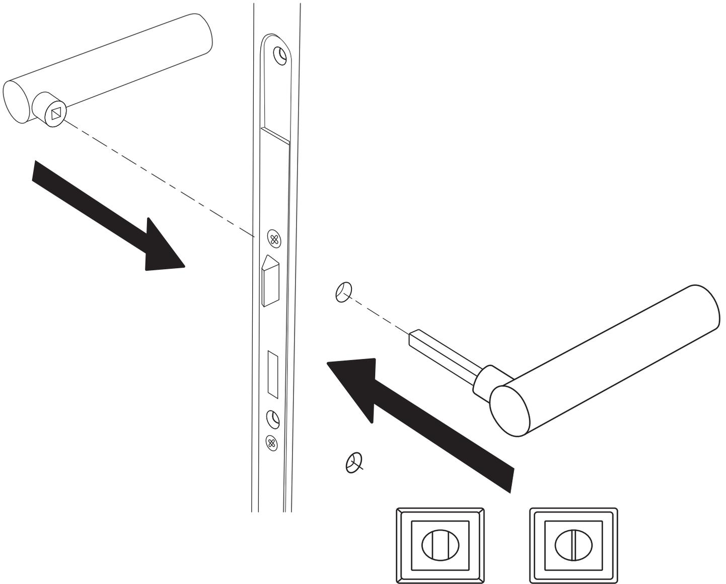
8) Fix the handle, then keyed mechanism and keyed cylinders into the pre-drillings
