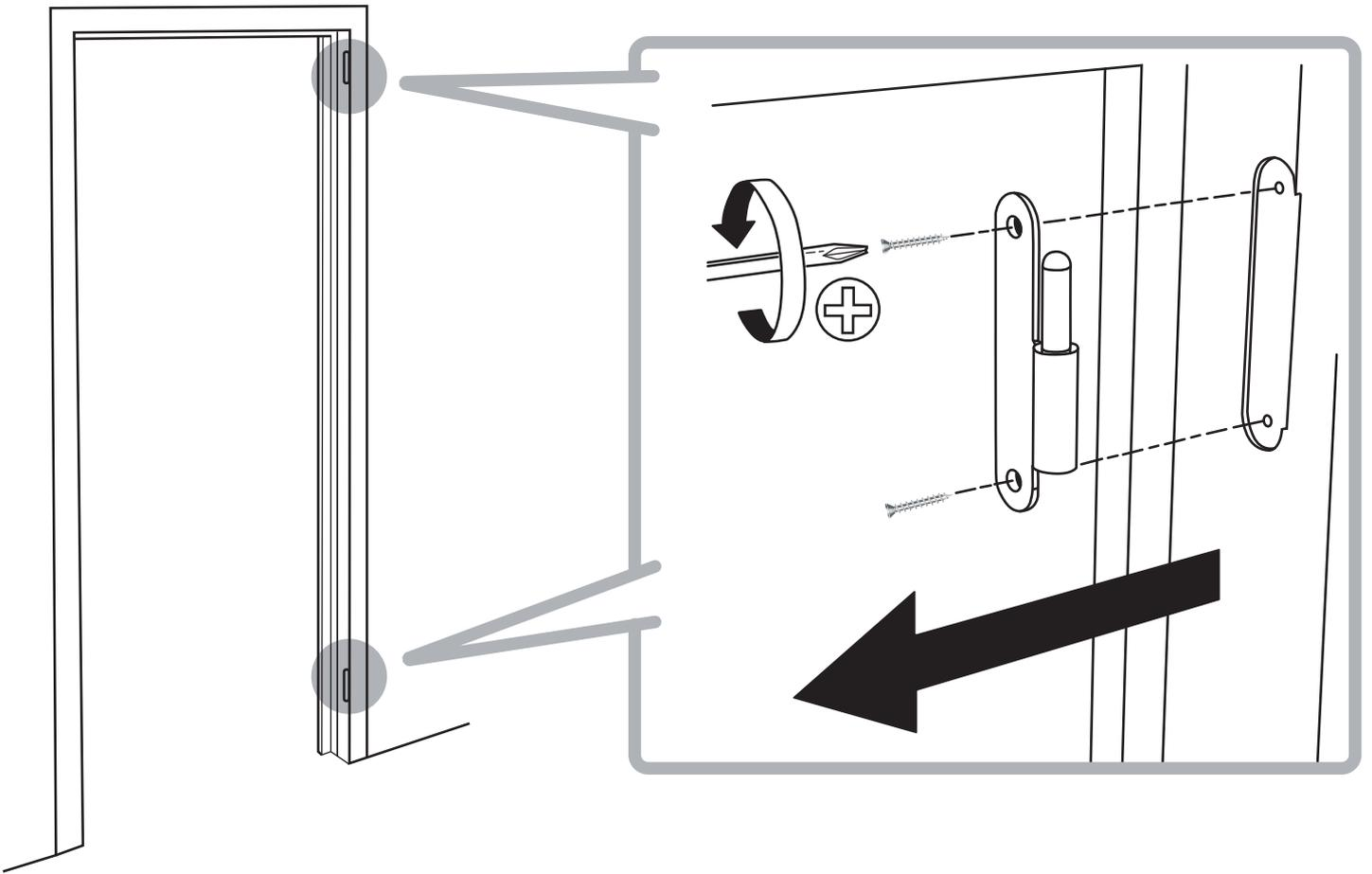
**3) Please, hang the door, after hardening for construction foam. Please note: different construction foams have different hardening levels. Read carefully the construction foam usage instructions!**
