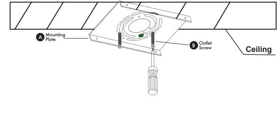
Attach mounting plate (A) to outlet box with outlet screws (B). Secure with Phillips head screwdriver or drill.
