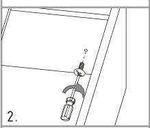
Secure two screws from the inside of the drawer using a Phillips screwdriver to tighten them to the outer slides.
