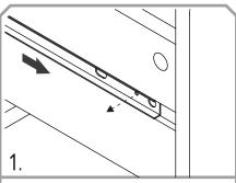
Extend the two outer slides of the runners so that they could align with the sides of the drawer. Make sure the pre-drilled holes from the drawer align with the screw holes of the outer slides.
