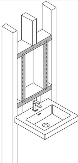
Frame the opening for the cabinet based on the measurements.
