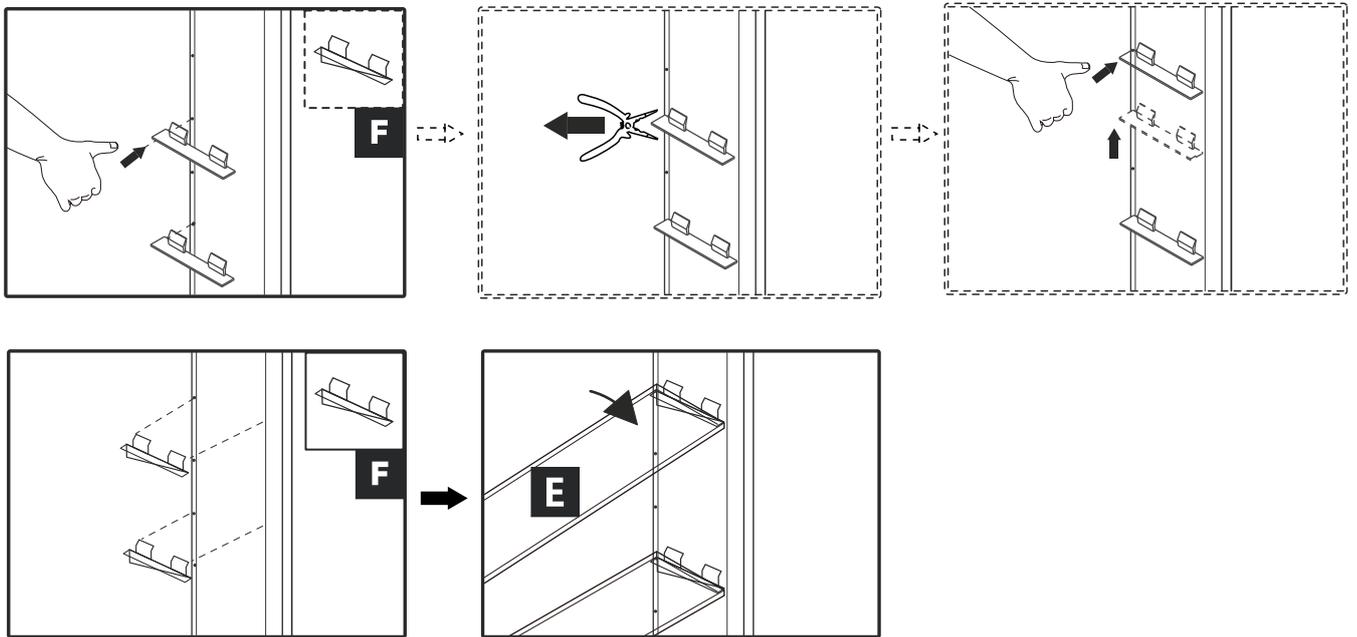
1. Insert clear snap in shelf clips (F) into holes on the sides of the cabinet.
