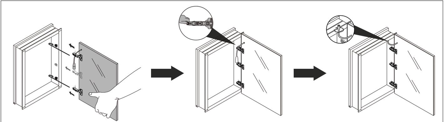
1. Slide the doors into place by pinching the end of the hinges.
