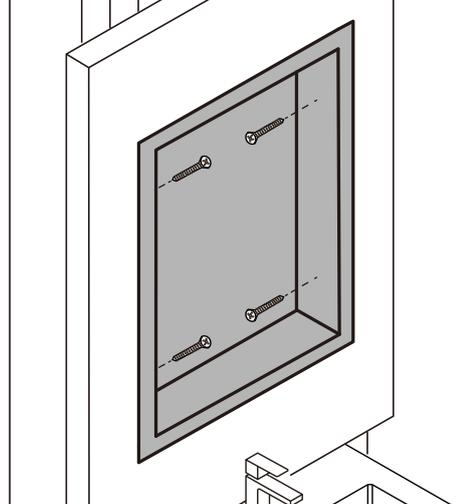
Affix using hardware screws into the studs.
