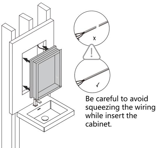
Be careful to avoid squeezing the wiring while insert the cabinet.
