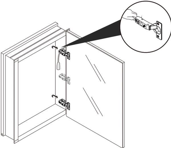
While supporting the door release (the lever under the hinge arm), slide the door off the frame.
