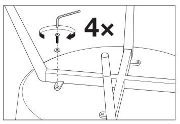
2. Fix the frame to the base using the allan screws combined with the metal rings. Secure the screws tightly before using the chair.
