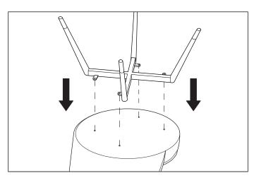
1. Align the frame of the legs with the screw holes on the base of the chair.
