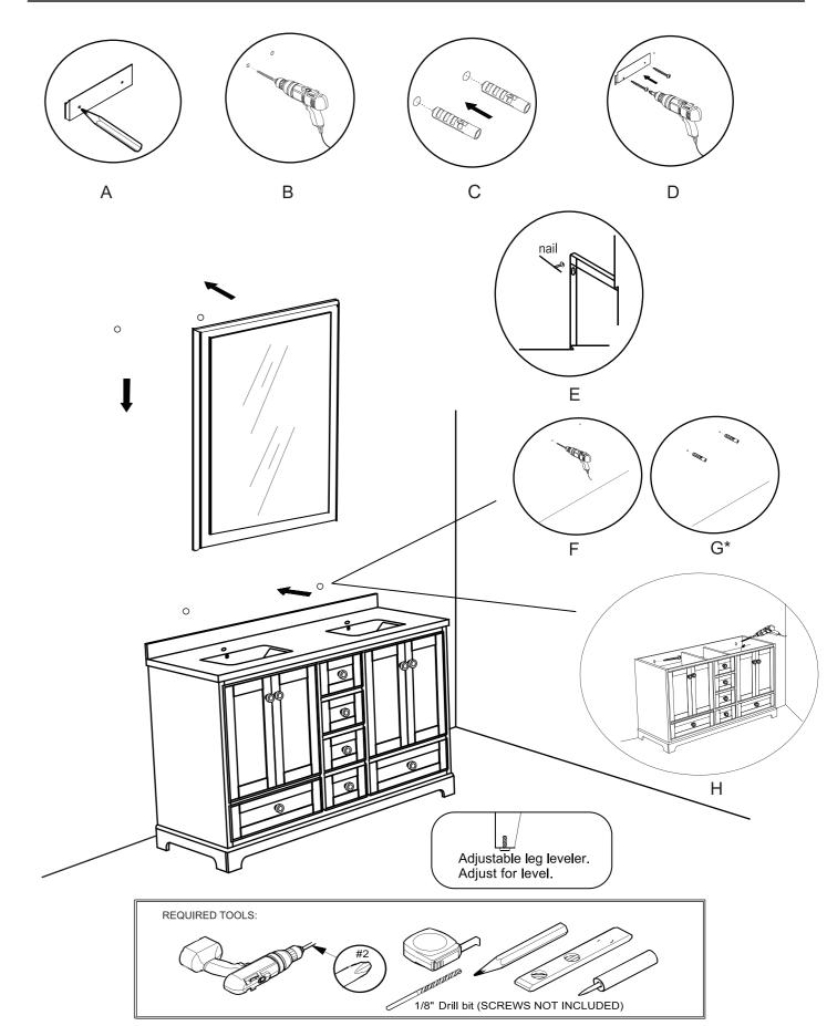
\*SECURE SCREW TO STUDS WHEN POSSIBLE
