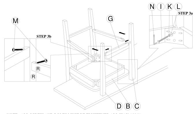
NOTE : ALL SCREW AND BOLTS MUST BE TIGHTENED ALL WAY (100%)
