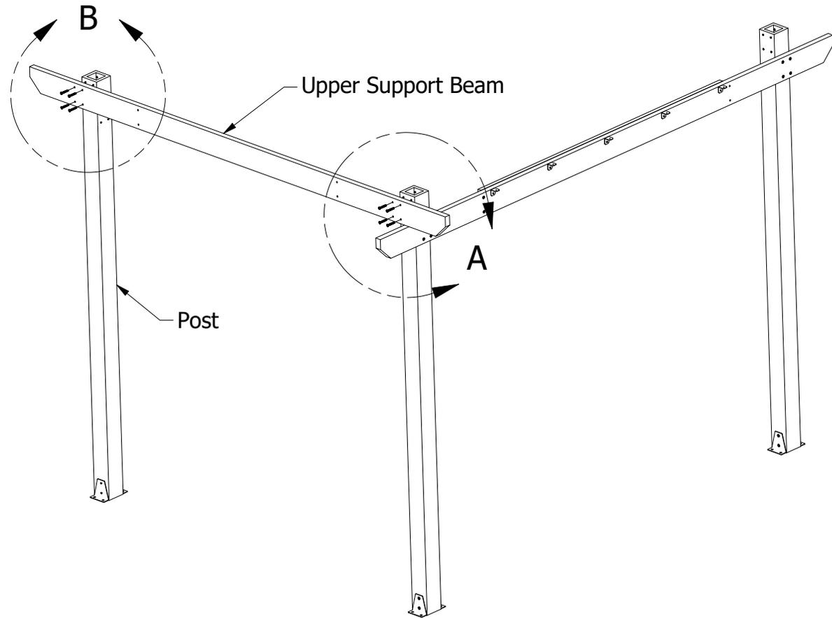
**9)** Lift an Upper Support Beam into Place as Shown. Support One End of the Beam Until Step 10, and Secure the Other End to the Arch Assembly from the Previous Step Using (4) "B" Bolts, as Shown in Detail "A".
