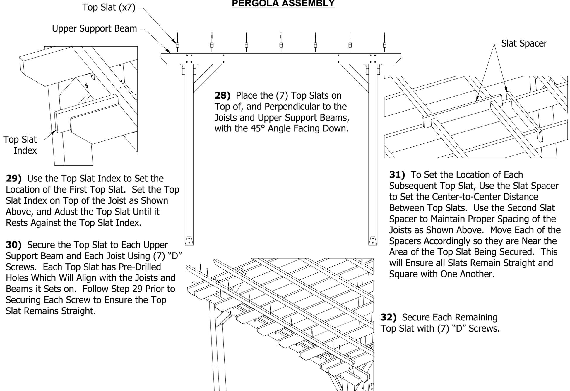
**28)** Place the (7) Top Slats on Top of, and Perpendicular to the Joists and Upper Support Beams, with the 45° Angle Facing Down.
