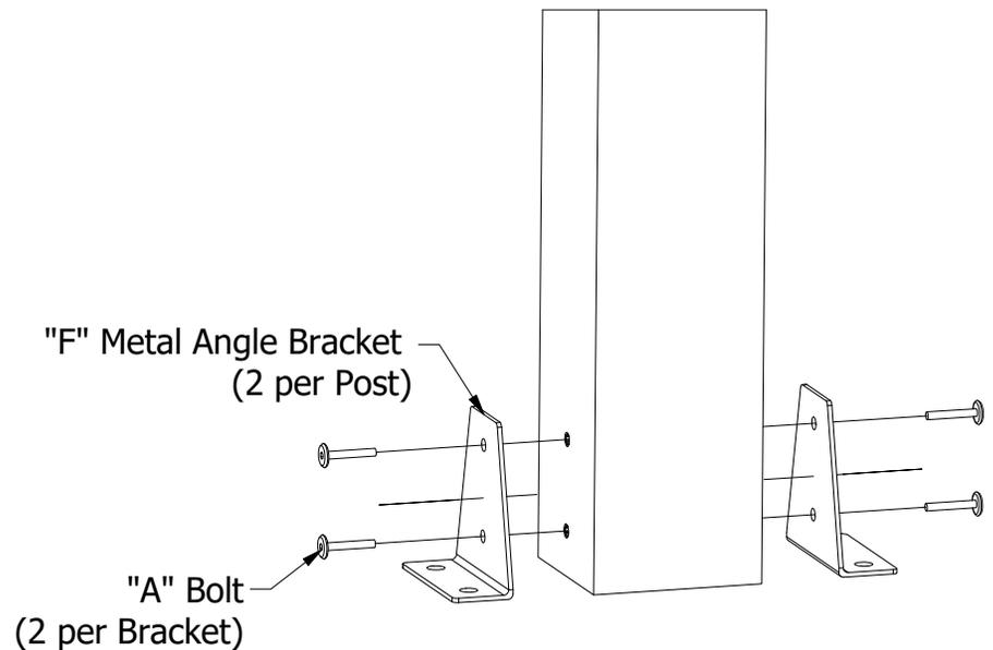
**3)** Attach (2) "F" Metal Angle Brackets to the Bottom of Each Post using (2) "A" Bolts as Shown. Holes in the Brackets will Align with Holes in the Posts.
