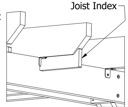
**26)** Use the Joist Index to Set the Distance Each Joist Overhangs the Lower Support Beam. Place the Joist Index Against the Lower Support Beam as Shown and Slide the Joist Until the 45° Cut Rests Against the Joist Index.
