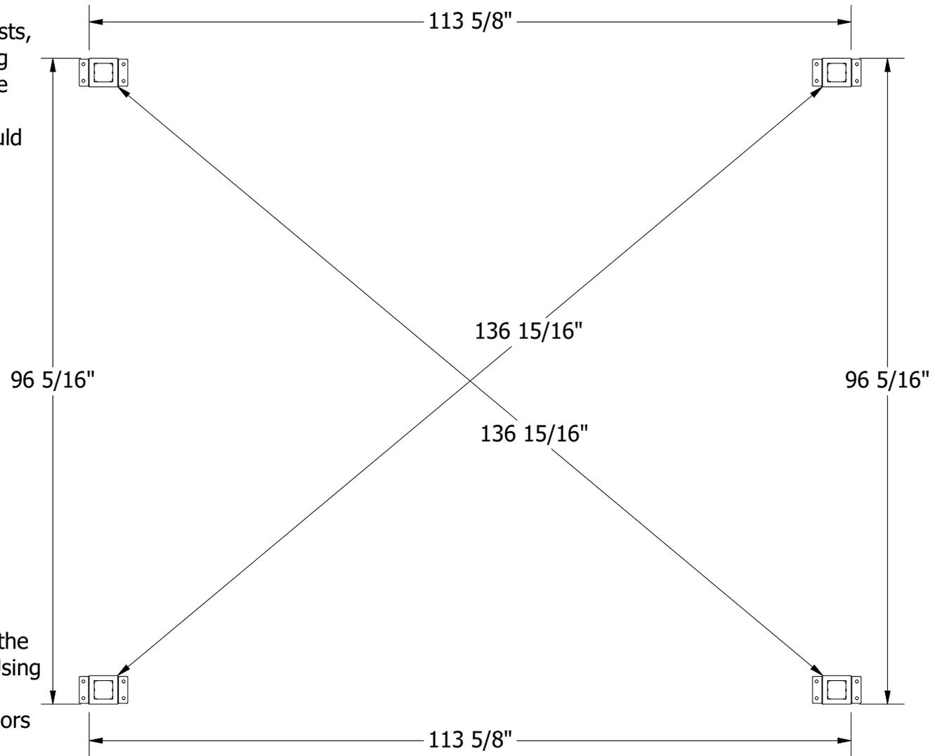
**23)** Once the Pergola Frame is Square, the Remaining (2) Posts can be Anchored. Using Anchors Appropriate for the Anchoring Surface, Secure the Posts Using (2) Anchors in Each "F" Metal Angle Bracket. The Brackets will Support Up to a  $\frac{5}{16}$ " Diameter Anchor.
