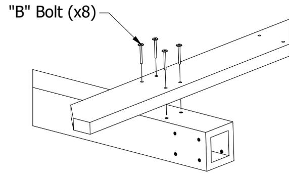
**6)** Attach the Lower Support Beam to Each Post Using (4) "B" Bolts.
