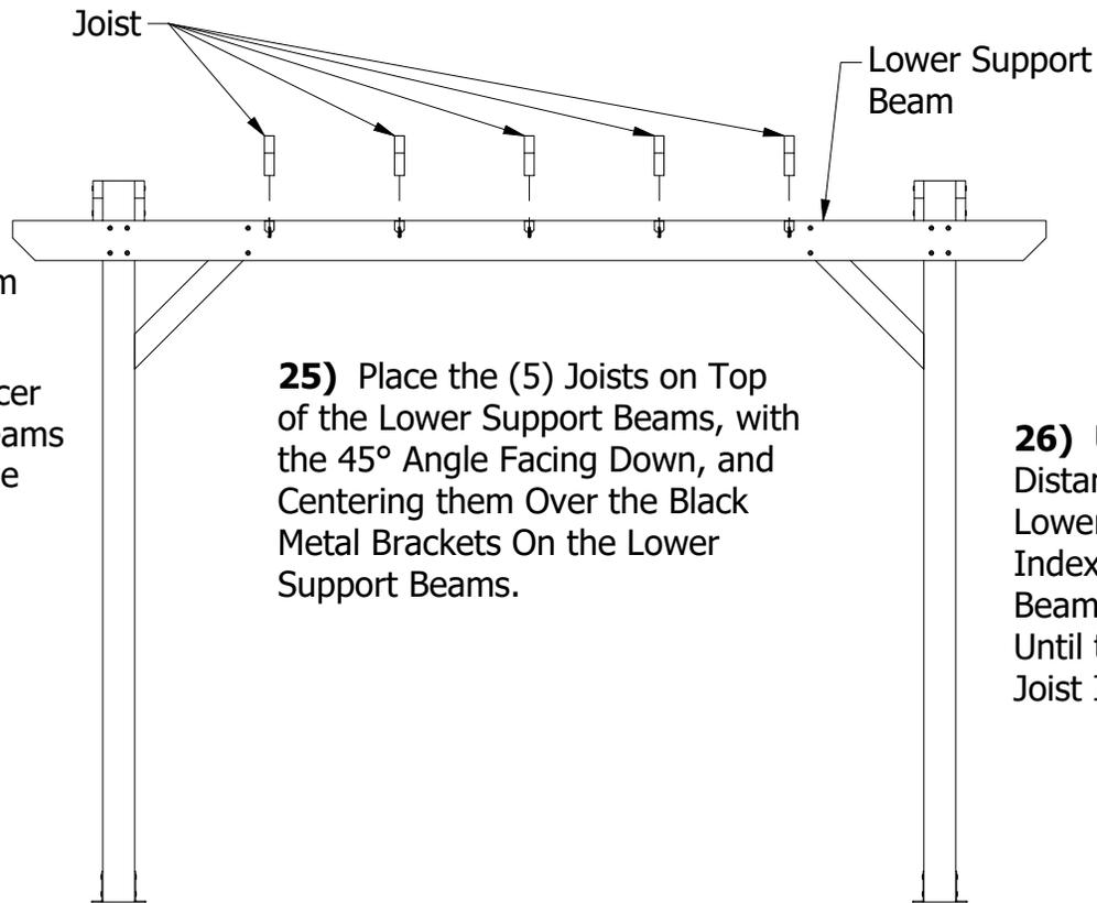
**25)** Place the (5) Joists on Top of the Lower Support Beams, with the 45° Angle Facing Down, and Centering them Over the Black Metal Brackets On the Lower Support Beams.
