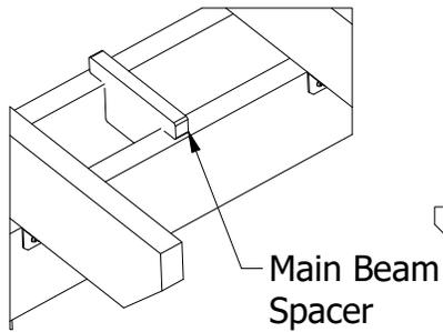
**24)** Place the Main Beam Spacer Between the Lower Support Beams as Shown Above to Maintain the Correct Beam Spacing.
