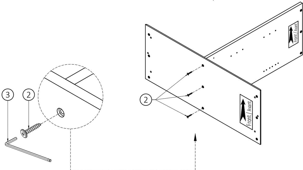
2. Use three Allen Key Screws (2) to attach Divider (C) through guide holes.
