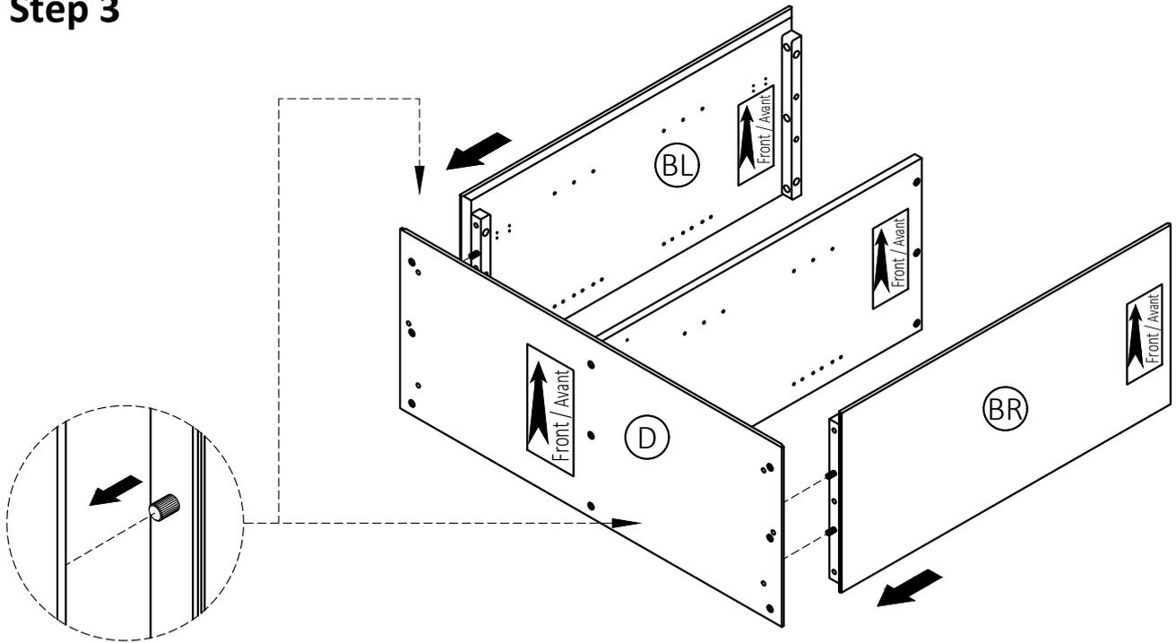
1. Align Wood Dowels with guide holes and attach Sides (BL), (BR) to Bottom Shelf (D).
