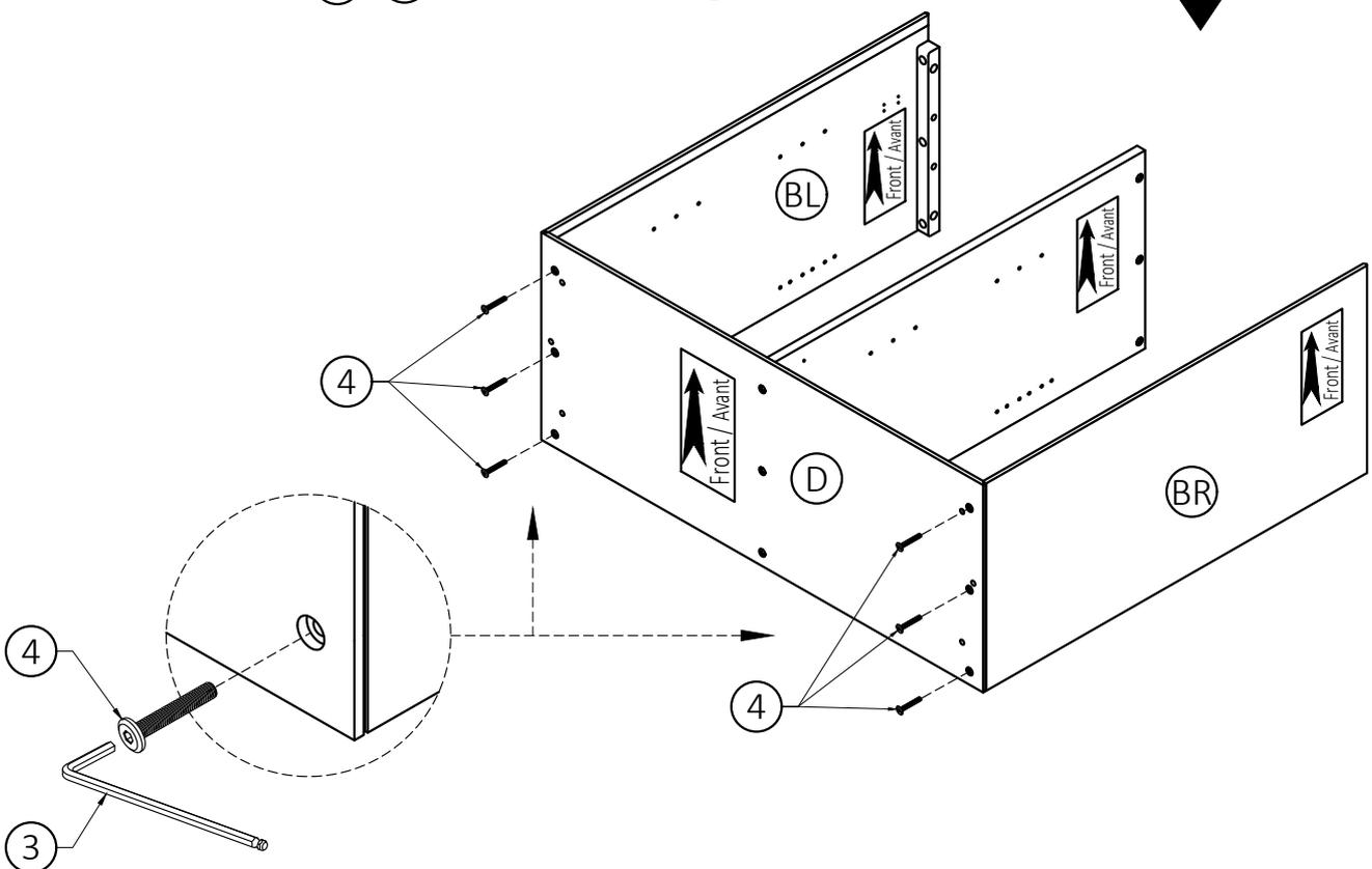
2. Use three Allen Key Bolts (4) to attach each Side (BL), (BR) through guide holes.
