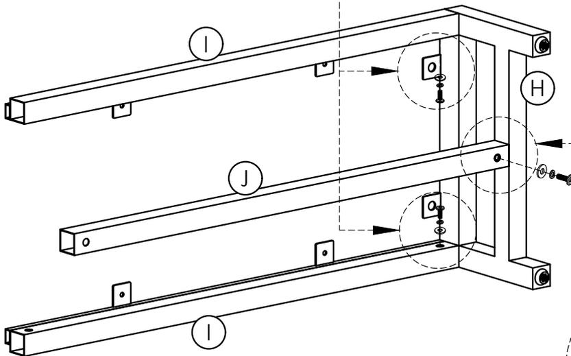
2. Use one Bolt (5), one Lock Washer (6) and one Washer (7) to secure each part (I), (J) with (H).
