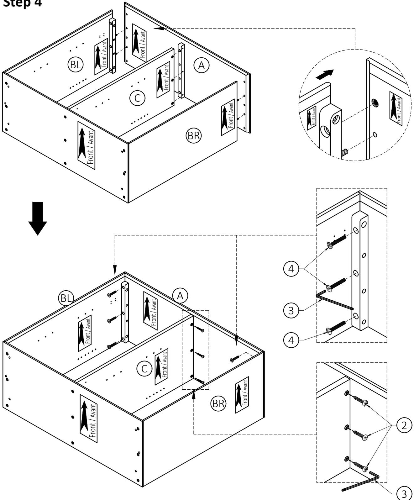
1. Align Wood Dowels with guide holes on Top (A) and attach Sides (BL), (BR) to Top (A).
