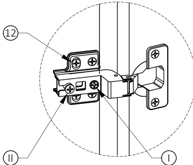
Tighten the Screw marked (II) to fasten hinge. The door may need to be adjusted so that all the spaces between the door and the unit sides are equal.
