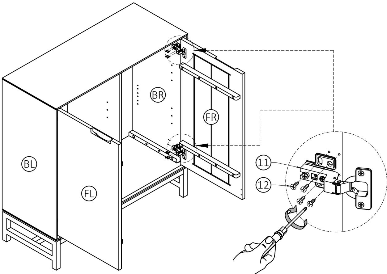
2. Attach Adjustable Hinges (11) on Doors (EL), (ER) to Sides (BL), (BR) using Phillips Screws (12) into pre-drilled holes on Sides (BL), (BR).
