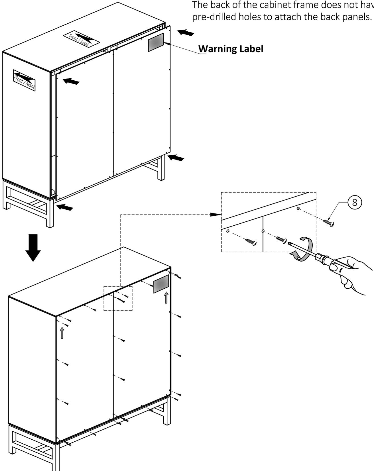
1. Attach the Back Panels (EL), (ER) to back frame using Phillips Screws Round Head (8) through guide holes from Back Panels.
