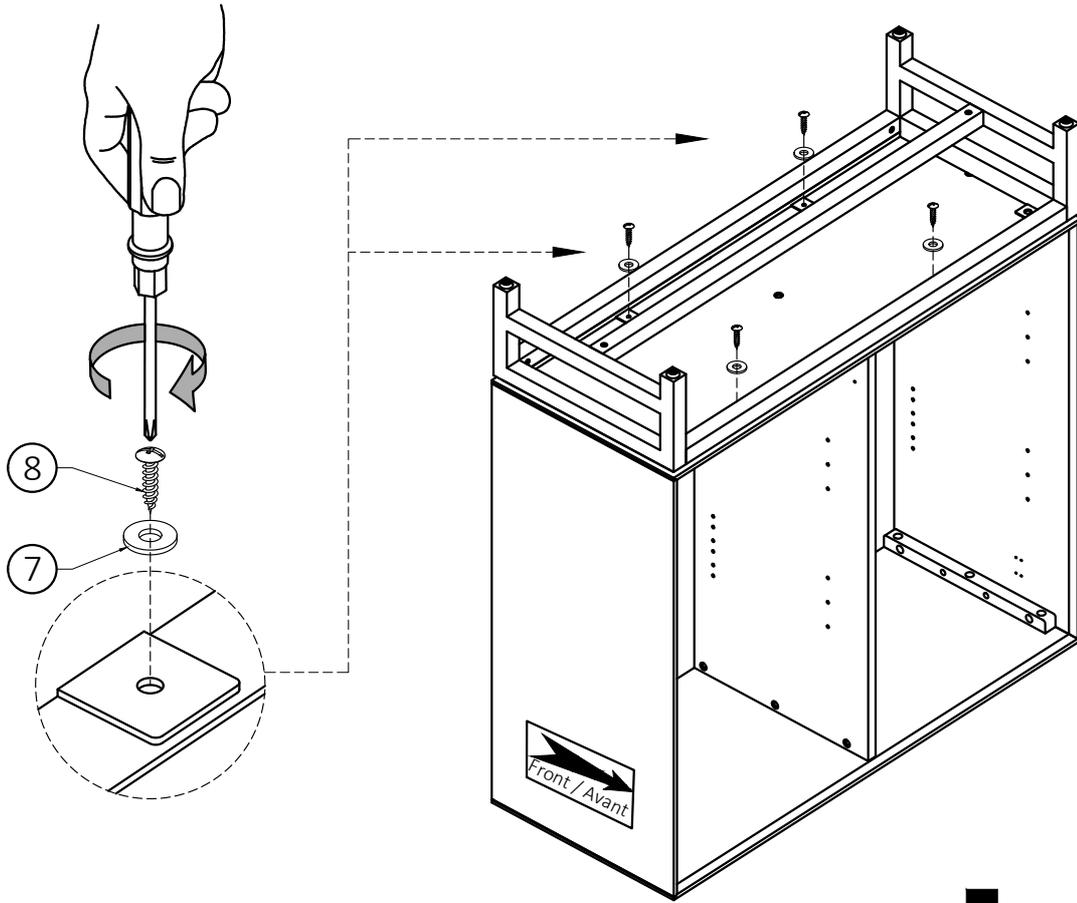
1. Use six Phillips Screws Round Head (8) and four Washers (7) to secure wooden frame and metal frame.
