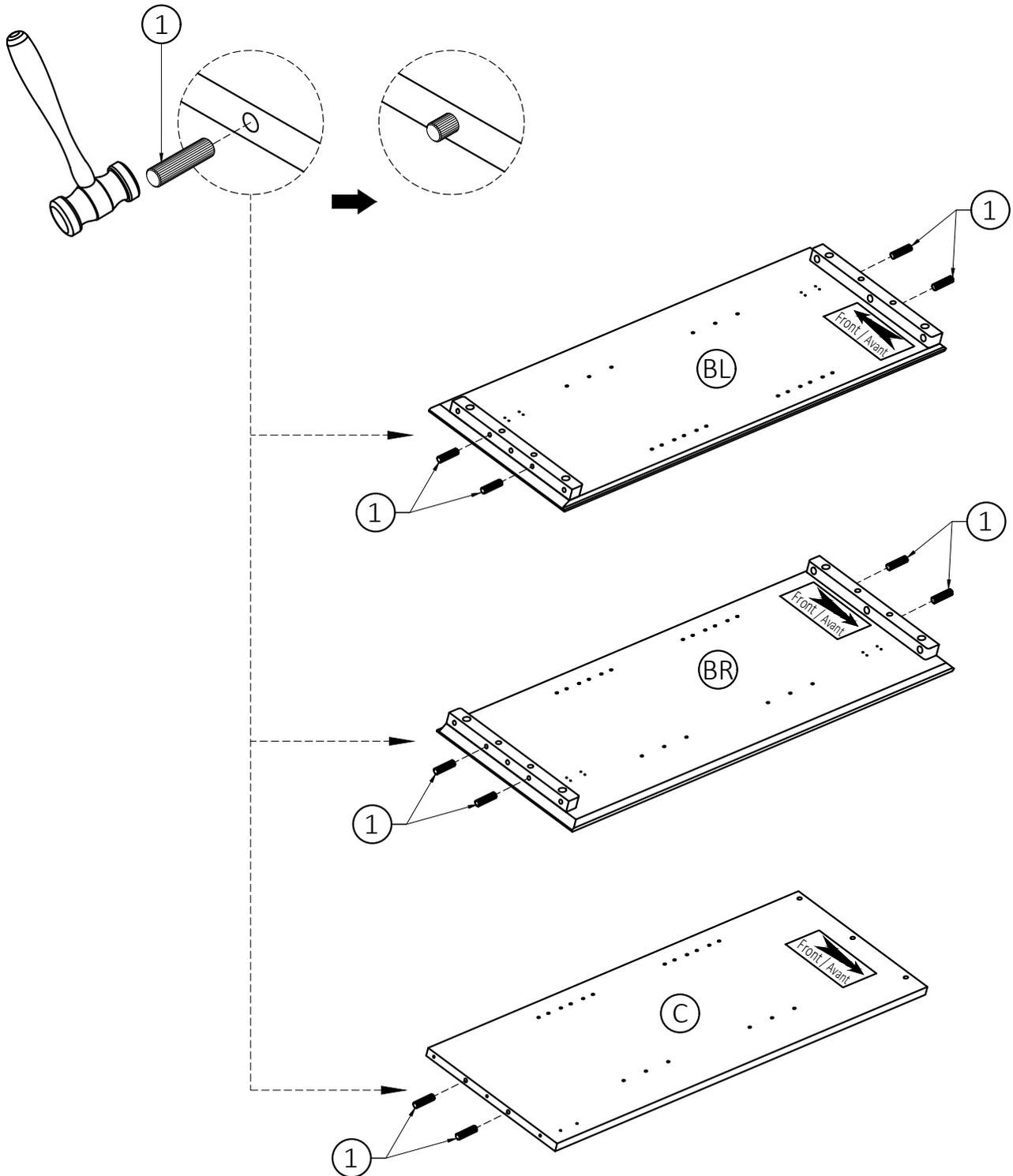
1. Insert Dowels ① into guide holes on Sides (BL), (BR) and Divider (C).
