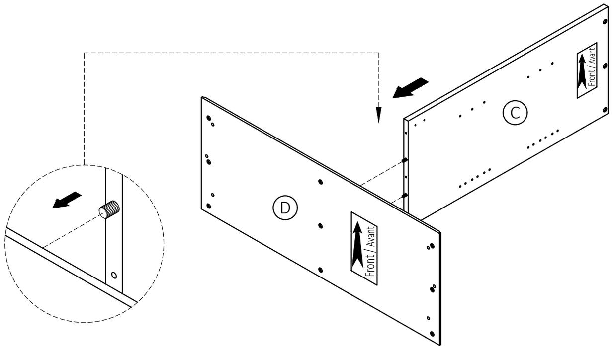
1. Align Wood Dowels with guide holes and attach Divider (C) to Bottom Shelf (D).
