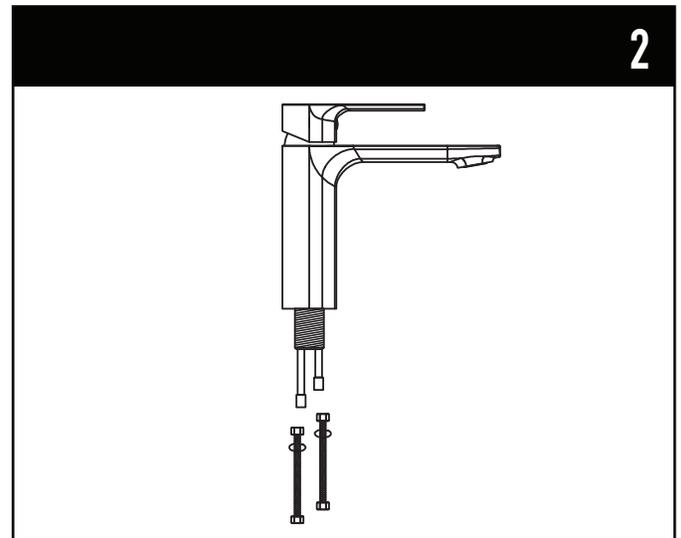
2. Connect flexible hoses to the brass pipes.
